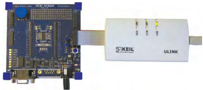
The Keil ULINK USB-JTAG Adapter connects to a wide range of evaluation boards. For more information refer to www.keil.com/ulink .
